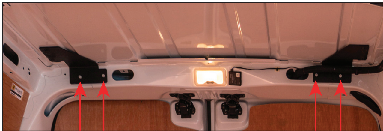
M6 1/4 TURN NUT INSERT LOCATIONS
