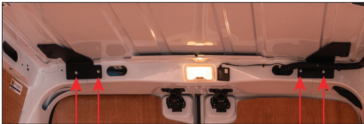
M6 1/4 TURN NUT INSERT LOCATIONS
